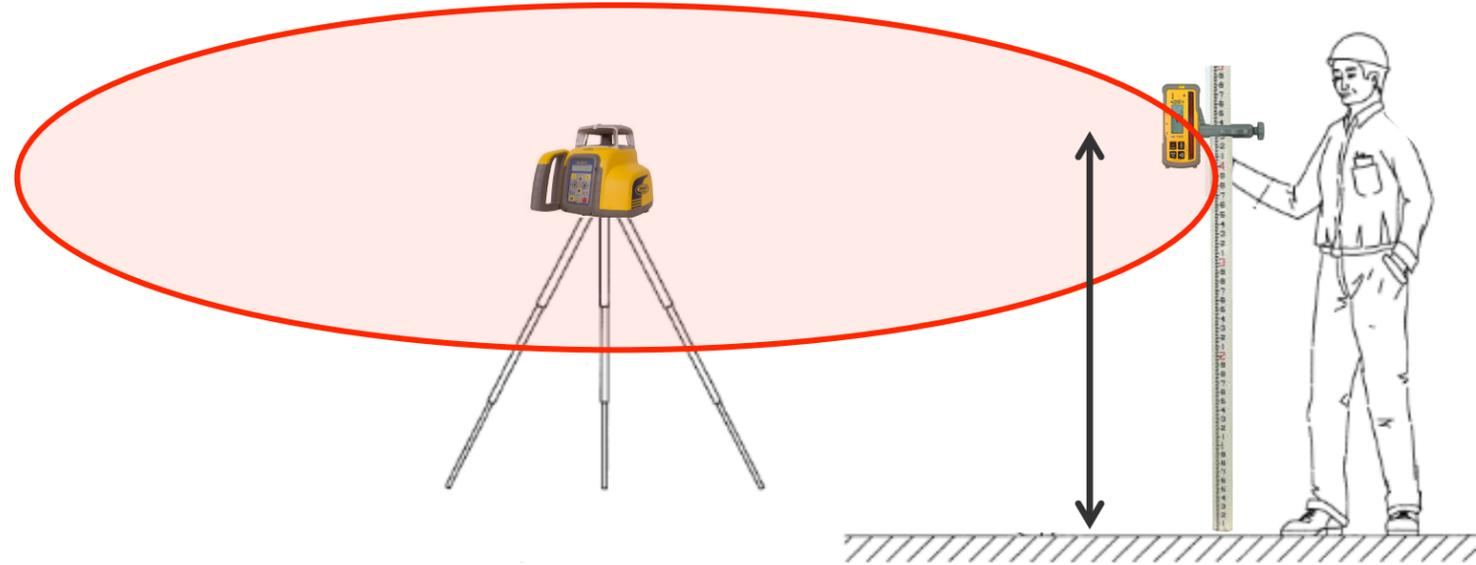
Laser receivers are used to level forms, concrete and dirt.
