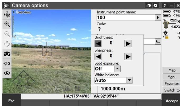
The following settings affect the image shown in the video display as well as images or scans captured using the instrument.
