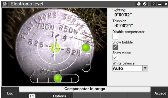
**NOTE** - To see movements in the instrument position reflected as expected in the video plummet display, orient the instrument so the handle is closest to the operator and the instrument is in the Face 1 position.
