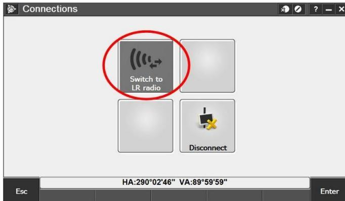
The radio settings are sent to the SX10 using the existing Wi-Fi connection and then applied when the controller connects to the instrument. The instrument will then change to LRR mode.
