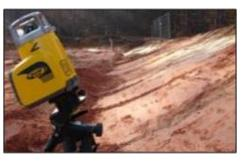
The M401 Tilting Base Adapter is a solid, reliable bracket that can be used for steep slope applications or with level-only lasers to manually accomplish grade. Formerly SECO part 4852-11.
