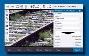
Based on the measurements, the current chainage and distance measurements in position and height to the track alignment are displayed directly in the field. When a main point is selected or a stake-out value is specified, the differences between the target value and the current position are displayed. The calculation can be done either horizontally or in a canted system. The interactive map view shows the track alignment with its main points and all measured points.
